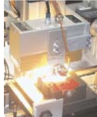
Preheating by infrared radiation of a halogen lamp with temperature control
