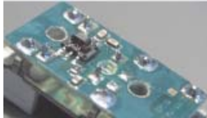
PCB with 9 solder joint in different locations distributed on the board
