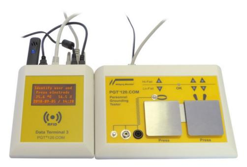
The Data Terminal DT3 can be use as a benchtop unit beside the PGT120.COM or with an additional wall mounting plate
