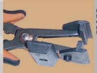
Extractor tool specially designed for the insertion and extraction of integrated circuits from 28 pins up to 40 pins
