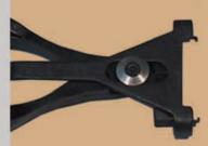
Extractor tool specially designed for the extraction of 32 pin PLCC type integrated circuits from the socket.
