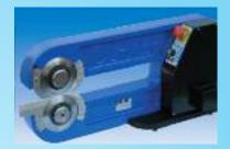
Motorized machine suitable to separate pre-assembled Electronic Board. Precise, reliable and safe. The PCB is manually fed between the lower and upper blades using the scoring as reference. By pushing the board horizontally, the blade rotation starts offering a sharp and accurate cut. The blade height is adjustable depending on the thickness of the PCB.
