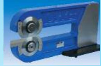
Manual machine suitable to separate pre-assembled Electronic Board. Precise, reliable and safe. The PCB is manually fed between the lower and upper blades using the scoring as reference. By pushing the board horizontally, the blade rotation starts offering a sharp and accurate cut. The blade height is adjustable depending on the thickness of the PCB. Upper and lower blades are also available titanium plated version
