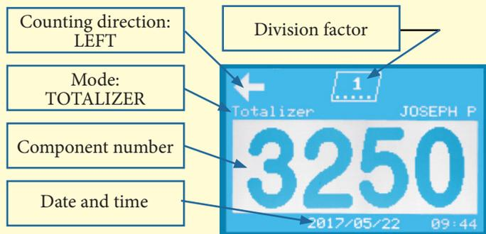
**2) PRESET MODE:** the desired component number is keyed on the keyboard and the counter automatically stops when it reaches the corresponding component
