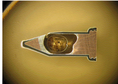
Cross section of a worn out Tip Lochbildung
